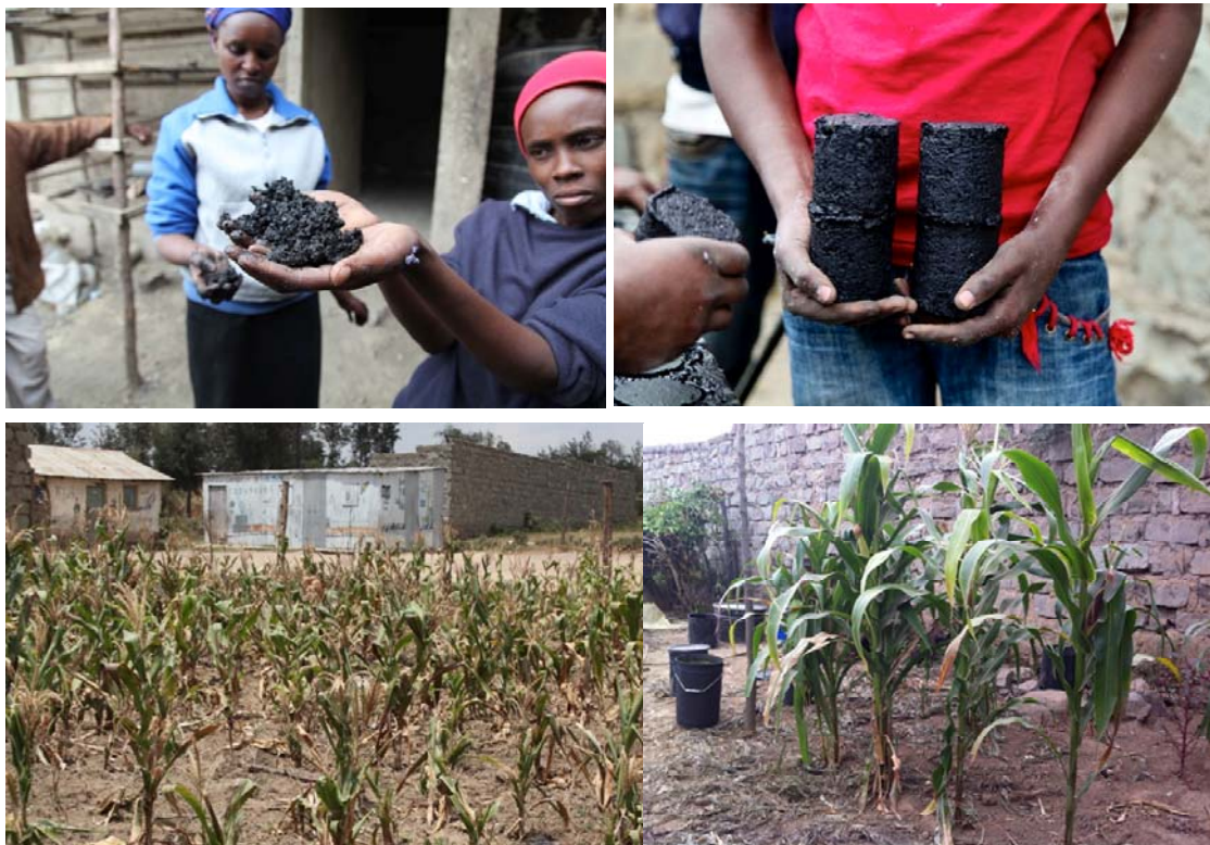
Figure 10: Manual fuel briquette production from human feces and charcoal dust in Kenya 2013.
